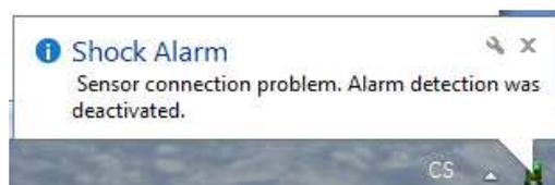
Sensor is not connected or sensor driver is not properly installed
